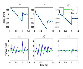
Fig. 3. Joint  $(\tau_1^m, \tau_2^m, \tau_3^m)$  and link side torque  $(\tau_1^l, \tau_2^l, \tau_3^l)$  values comparison made between the virtual model  $(mod_{ad})$  and numerically computed model  $(mod_3)$  using (1), for a pre-defined joint motion.
