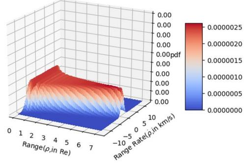
Figure 1: Gaussian Mixture Admissible Region representation, using 300 components, according to [4].
