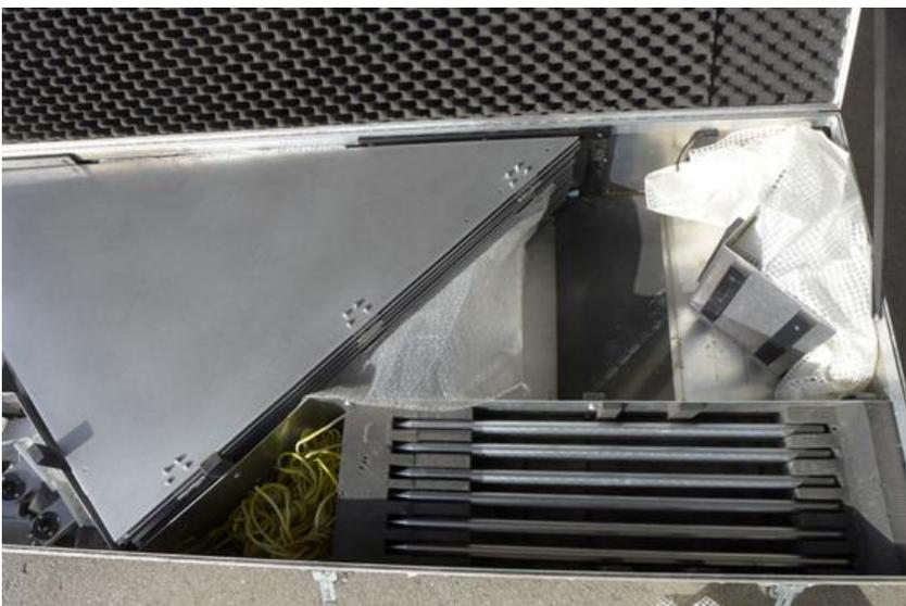
Figure 2-4: Newly built foldable radar reflectors of 95cm inner leg-length inside transport box.
