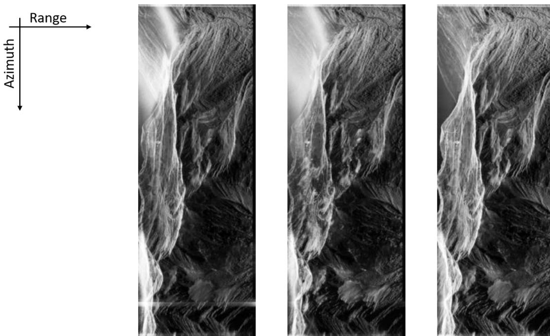
Figure 5-3: For comparison an F-SAR single pass, single-look complex (SLC) image (resolution: 0.5 m x 0.5 m; samples: 24320 x 7536) of flight 2 with track 10 for different polarisations. From left to right: HH, HV, VV.
