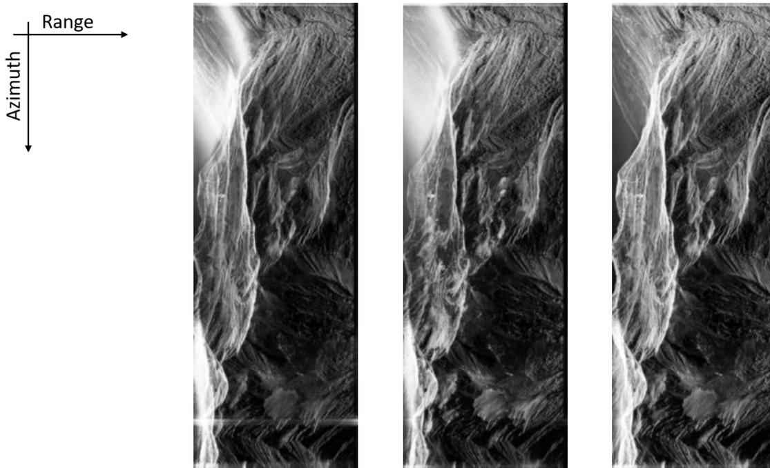
Figure 5-2: Simulated single-look complex (SLC) product of geosynchronous SAR (resolution: 0.5 m x 0.5 m; samples: 24320 x 7536) from F-SAR data of flight 2 with track 10 for different polarisations. From left to right: HH, HV, VV.
