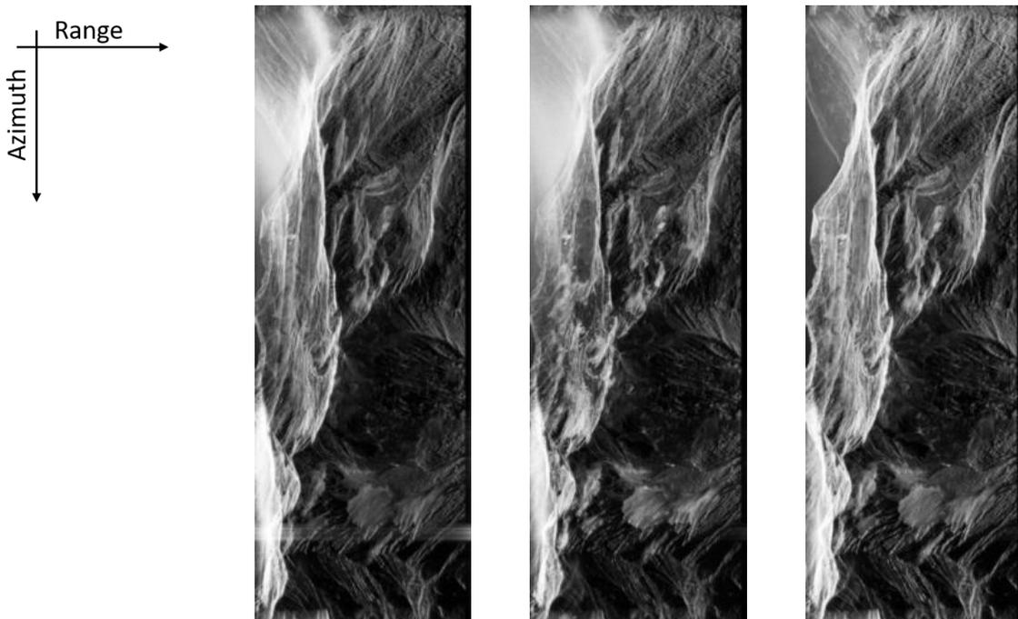
Figure 5-7: For comparison an F-SAR single pass, single-look complex (SLC) image (resolution: 0.5 m x 0.5 m; samples: 24320 x 7536) of flight 5 with track 10 for different polarisations. From left to right: HH, HV, VV.
