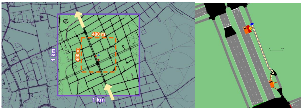
Figure 6: Left: violet square: the simulated area, orange square: the measuring range, blue triangle: the user request, red circles: the stop candidates, yellow arrows: the shuttle route. Right: blue triangle: the user request, dotted lines: the user's paths to the stops
