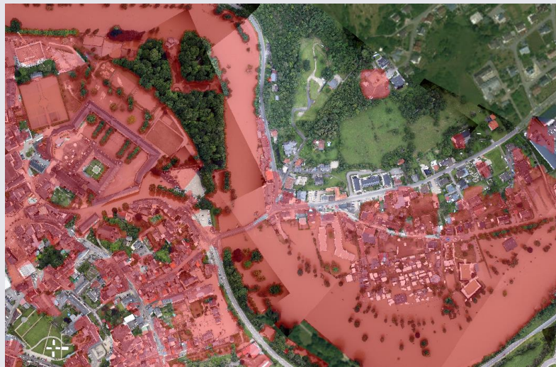
Raw output of flood detection by means of Deep learning
