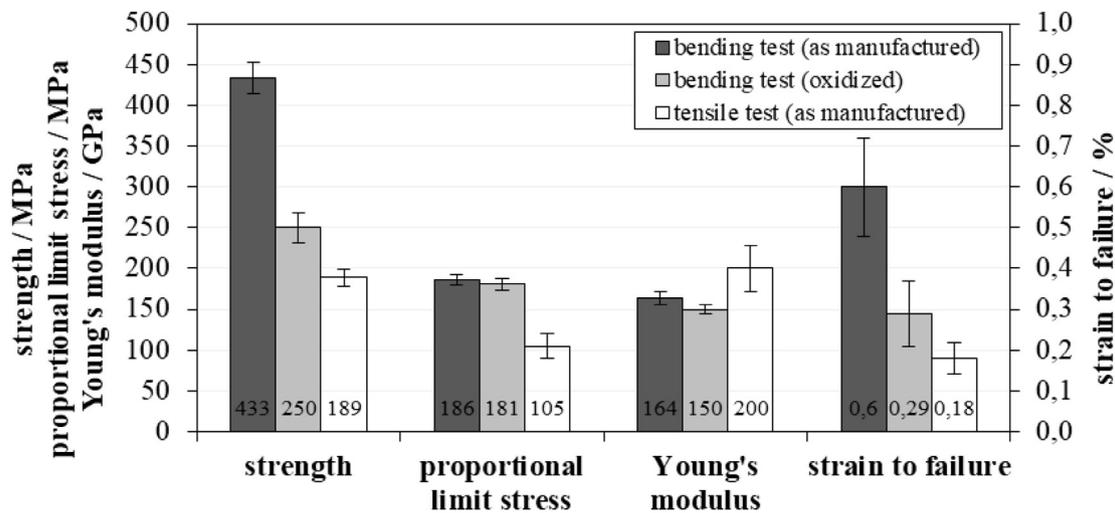
Fig. 8. Comparison of the mechanical properties of the hybrid composite manufactured in approach #3 in four-point bending testing before and after oxidation, as well as in tensile testing.
