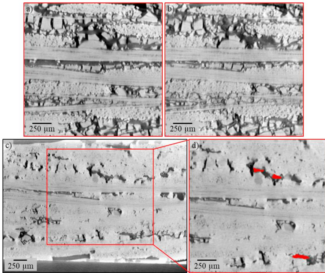
**Fig. 5.**  $\mu$ CT scans at the same area of one sample of (a) after 2 cycles of polymer infiltration and pyrolysis, (b) after the infiltration of phenolic resin and pyrolysis (c) and (d) after melt infiltration with liquid silicon. Residual carbon after siliconization is highlighted in red. (For interpretation of the references to colour in this figure legend, the reader is referred to the Web version of this article.)
