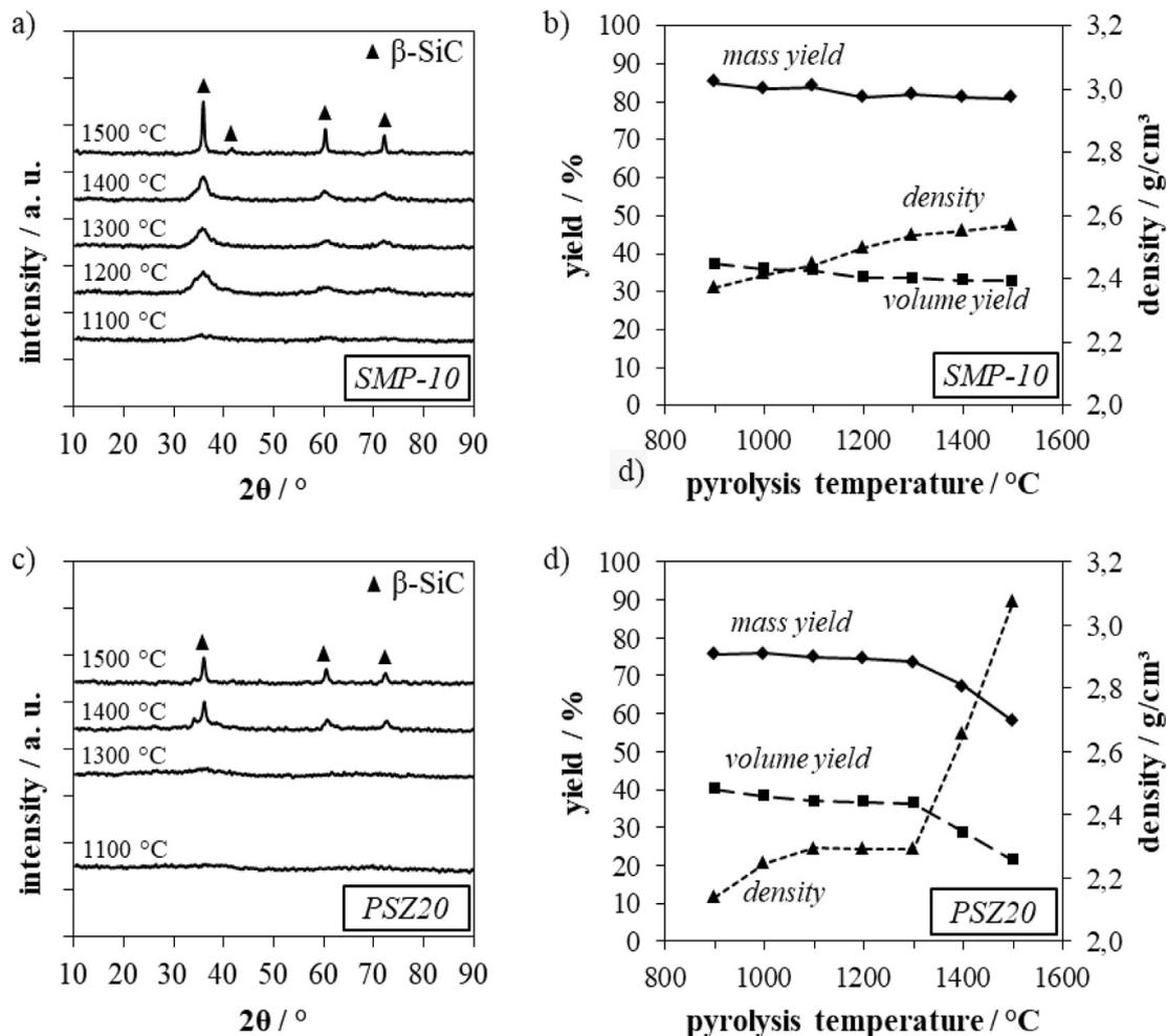
**Fig. 2.** Characterization of the polymeric precursors SMP-10 and PSZ20. Pyrolysis of cured sample material was carried out in argon atmosphere for 10 h. Crystallization of SMP-10 and PSZ20 (a) and (c). Mass yield, density and volume yield of SMP-10 and PSZ20 (b) and (d).
