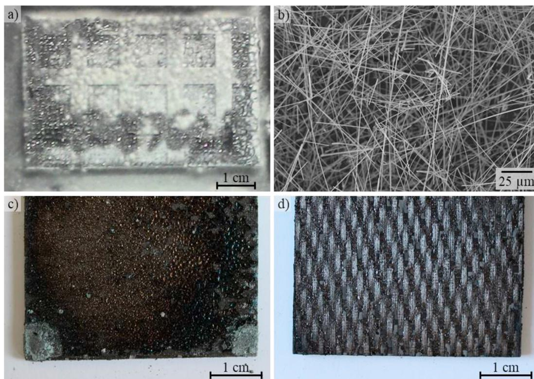
**Fig. 3.** Whisker formation after pyrolysis of phenolic resin in nitrogen atmosphere (a). SEM image of  $\text{Si}_3\text{N}_4$  whiskers (identified by XRD) (b) [23]. Reduced whisker formation when pyrolyzed in Ar instead of  $\text{N}_2$ , water and oxygen contact was avoided, too (approach #1) (c). No whisker formation was observed when polycarbosilane precursor SMP-10 was used in approach #2 (d).
