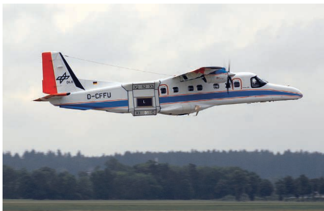
Figure 1. Photograph of the DLR research aircraft Dornier Do-228-212 showing the SAR antenna positions (© DLR).
