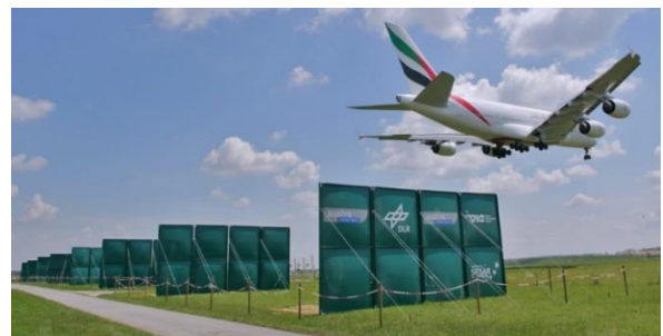
Fig. 3: Overflight of A380 of one of the experimental plate lines installed at runway 16 of Airport Vienna.
