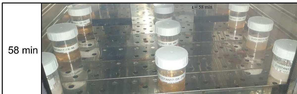
Figure 21: Varying pre-gelation progress of RFB sols after 58 min at 60 °C. Containers are placed on various positions.
