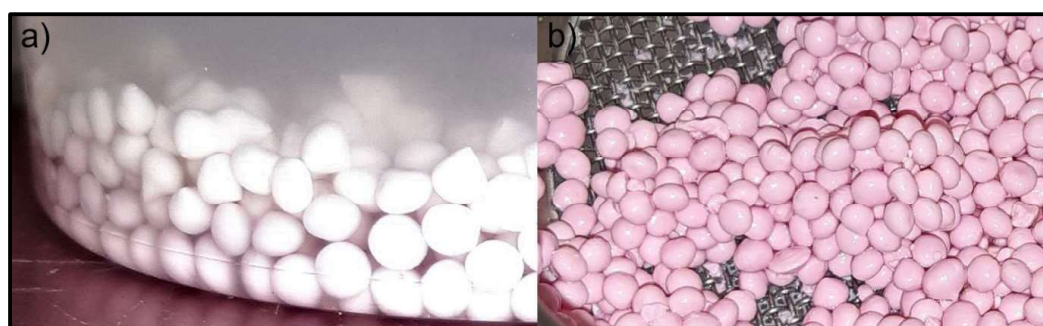
Figure 23: Color of RF aerogel microbeads: a) right after dropping and b) filtered after few minutes in the gelation bath.
