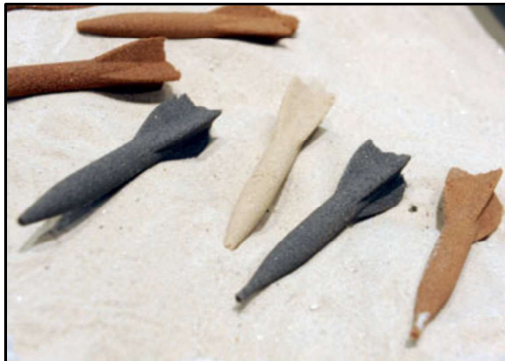
Figure 7: Sand casting cores made with 1.5% aerogel additive. Brown: RF aerogel, buff colored: silica aerogel and black: carbon aerogel. [24]
