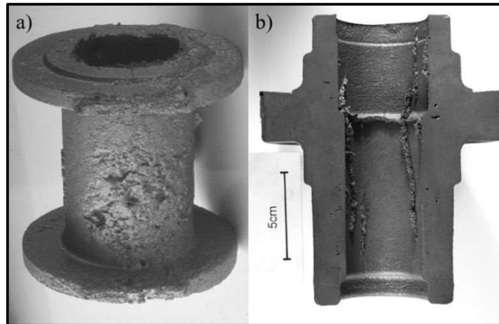
Figure 1: Common defects in the form of a) blow holes [9] and b) veining [10] , occurred in casting parts made by a sand casting process.
