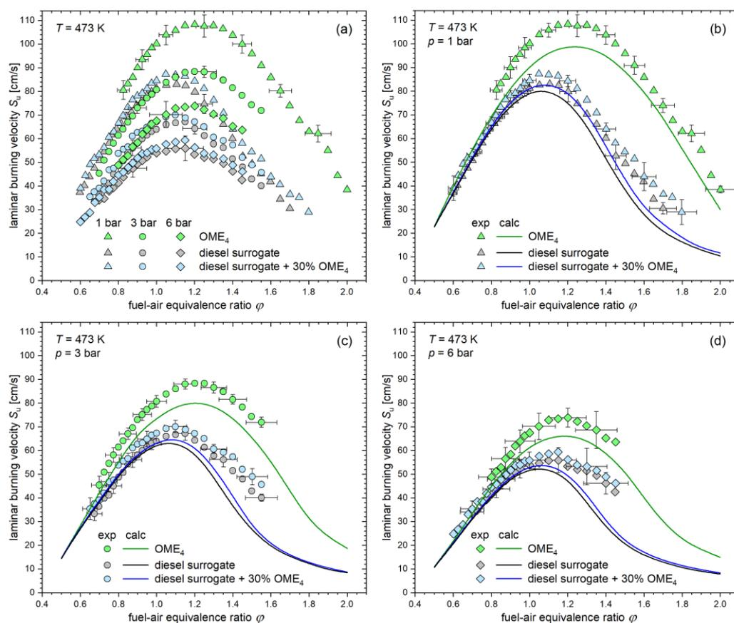
**Figure 8.** Results of the measured laminar burning velocities at  $T = 473$  K of the diesel surrogate, neat OME<sub>4</sub>, and diesel surrogate and 30% (*w/w*) OME<sub>4</sub> (a) and comparison between the experimental data and the calculated laminar flame speeds for 1 bar (b), 3 bar (c), and 6 bar (d).
