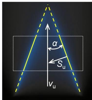
**Figure 6.** Relation between the laminar burning velocity ( $S_u$ ), the cone angle ( $\alpha$ ), and the gas flow velocity ( $v_u$ ) of a laminar premixed conical flame.
