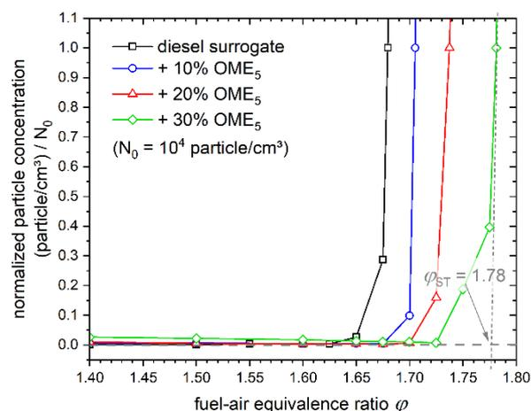
**Figure 4.** Normalized particle concentrations for the diesel surrogate and the surrogate-OME<sub>5</sub> mixtures (percentage given in mass fraction) showing the extrapolation to the soot threshold ( $\phi_{ST}$ ). The grey dashed tangent line indicates the maximum gradient of the increasing particle concentration for the mixture of the diesel surrogate with 30% (*w/w*) OME<sub>5</sub> and is extrapolated to the base line where the intersection gives the value for  $\phi_{ST}$ .
