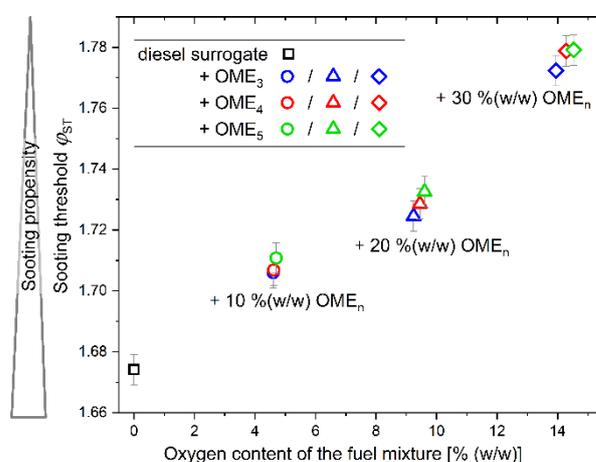
**Figure 7.** Results of the determined sooting propensities using the soot threshold ( $\varphi_{ST}$ ) as indicator.
