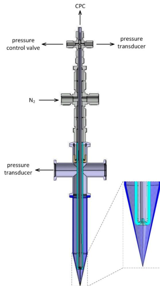
**Figure 3.** Scheme of the sampling unit used for the measurement of the sooting propensity (inlets, as they were not labeled, were closed during the measurement); CPC—condensation particle counter.
