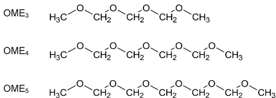
**Figure 1.** Molecular structures of OME<sub>3</sub>, OME<sub>4</sub>, and OME<sub>5</sub>.
