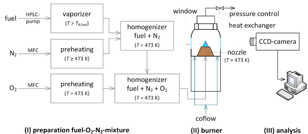
**Figure 5.** Scheme of the experimental set-up for the measurement of the laminar burning velocity of a conical laminar flame. The temperature of the nitrogen preheating depends on the final boiling of the fuel mixture but is at least 473 K; HPLC—high performance liquid chromatography, MFC—mass flow controller,  $T_{B,fuel}$ —final boiling point of the fuel mixture.
