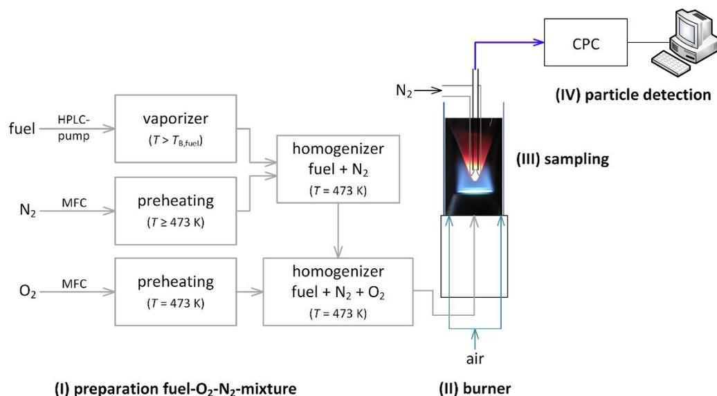
**Figure 2.** Scheme of the experimental set-up for the measurement of particle concentration in the exhaust gas of a plane-laminar flame. The specific preheating temperature of nitrogen is at least 473 K, subjected to the final boiling of the fuel mixture; CPC—condensation particle counter, HPLC—high performance liquid chromatography, MFC—mass flow controller,  $T_{B,\text{fuel}}$ —final boiling point of the fuel mixture.
