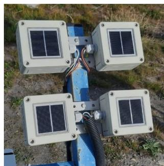
Figure 1: Two pairs of PV reference cells (PVRC) mounted at CIEMAT's Plataforma Solar de Almería, Spain. The left pair uses textured glass, the right pair smooth glass. The upper row is cleaned and the lower row is soiled. The right pair is used in this study
