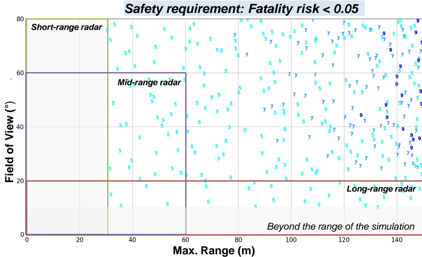
**Using a *single radar* (regardless of radar type), the safety requirement (fatality risk < 0.05) is met when ego-vehicle velocity is less than 50km/h**
