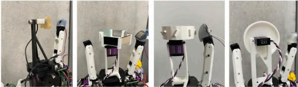
**FIGURE 6 |** Testbeds for verification of the tactile sensors on the CLASH 2F. **From left to right**, testbeds for: sensibility depending on stiffness, sensibility depending on surface materials, edge detection, and slippage detection.
