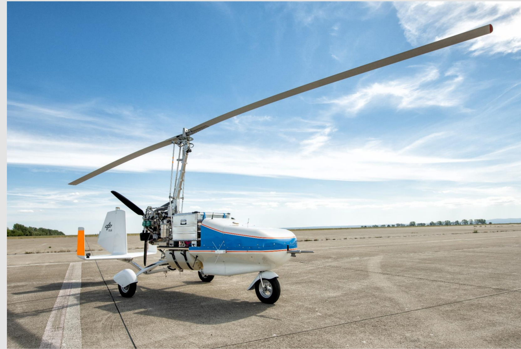
Figure 1: Unmanned cargo gyrocopter ALAAdy-Demonstrator capable of carrying up to 50 kg of payload
