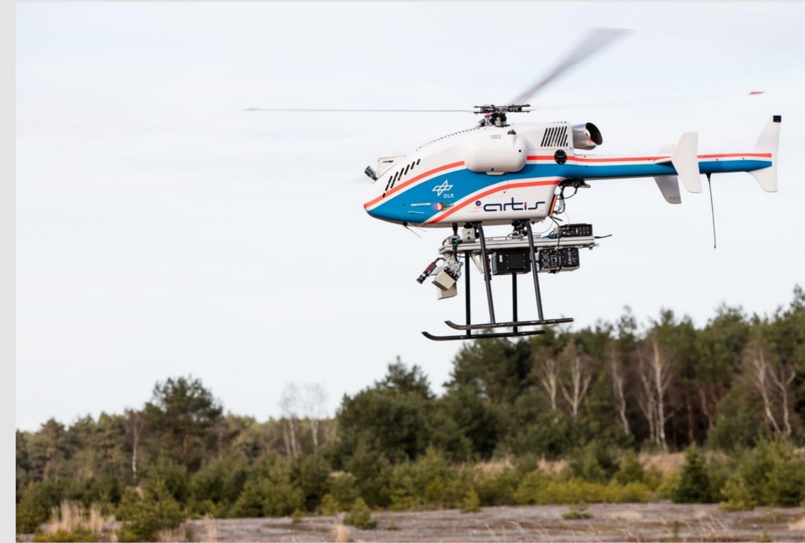
Figure 2: Unmanned helicopter superARTIS equipped with LIDAR and optical sensors for environment perceptions in autonomous flight
