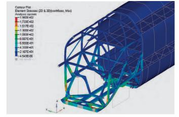
Simulations can be used to test the structural loads on the body of a train. The red areas show highly stressed components.
