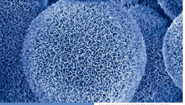
A new biopolymer aerogel developed by DLR scientists in a laboratory experiment. The spherical and filamentary structures are created when chitosan is combined with a thermoset.
