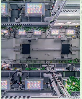
View of the water-cooled LED systems from below. These shine light on the plants in a precisely coordinated day-night rhythm.
