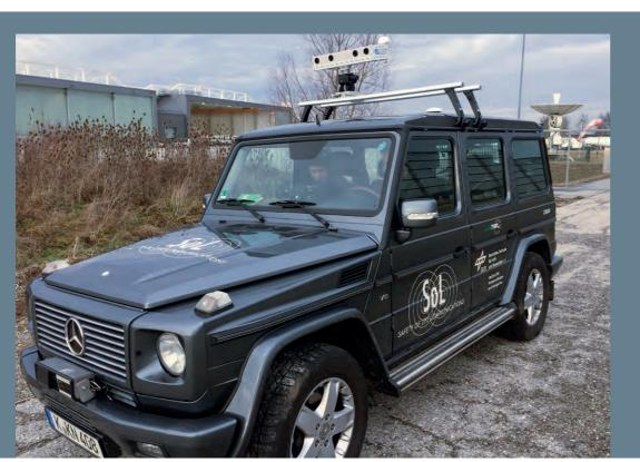
autonomous driving and surveying of road infrastructure, as shown here with a resear vehicle from the DLR Institute of Communications and Navigation.
