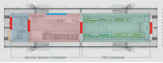
The EDEN ISS Service Section container houses an airlock (shown in blue) for changing Antarctic clothing. Next to it (red) is the area for the atmosphere management system, the nutrient supply system, the thermal regulation system and the data handling system. The Future Exploration Greenhouse (green) container generates fresh produce in 12.5 square metres.
