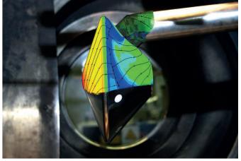
Experimental and numerical simulations of the entry of a landing capsule into the Martian atmosphere.
