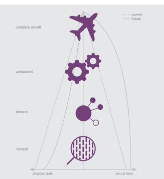
This test pyramid from the aeronautics sector shows the development steps from initial material tests to the design and testing of individual elements and components and then on to the complete aircraft system. In future, physical verification of certifications will be increasingly supplemented by virtual tests, and perhaps even replaced by them in the longer term.
