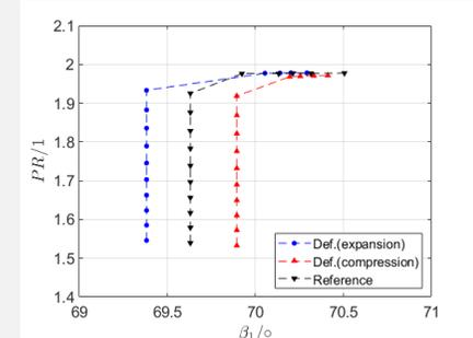
First results show that even small deformations at the blade's tip can lead to a positive influence on the blade's performance under transonic conditions.
