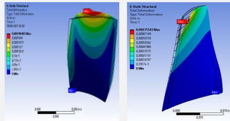
The figure above, left, illustrates an example for the total deformation that can be achieved for a blade with two integrated large surface Macro Fiber Composite (MFC) piezo-actuators, one on the pressure side and one on the suction side, both actuating in the chordwise direction, the one on the pressure side set on compression mode and the one on the suction side on expansion mode and maximizing camber.
