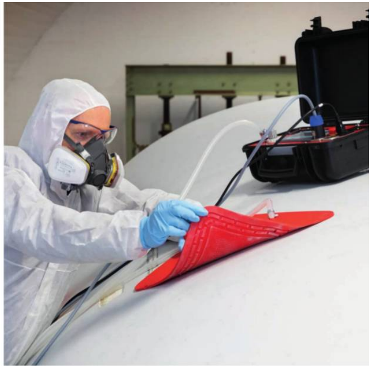
Repair test on the outer skin of a rotor blade with the vacuum heating mat developed at DLR
