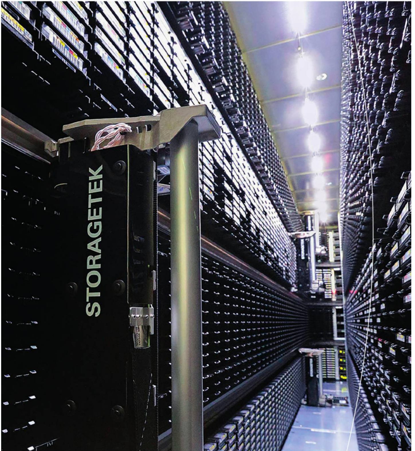
DLR's German Remote Sensing Data Center (DFD) operates the German Satellite Data Archive (DSDA) in Oberpfaffenhofen. DFD is setting up a processing and archiving centre on behalf of the European Space Agency (ESA): The robot-based DSDA stores, among other things, the image data acquired by the Copernicus satellites Sentinel-1 and Sentinel-3.
