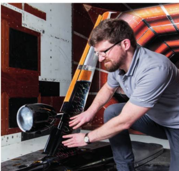
The effect of 'pulsed discharge' for active flow control was measured on a model of a complete wing in the Cryogenic Wind Tunnel Cologne, which is operated by the German-Dutch Wind Tunnels foundation. For this purpose, small actuator chambers were installed in the leading edge of the model, from which compressed air can be blown through six small double slots onto the wing surface connected through a small tube to the external energy source. Vlad Ciobaca from the DLR Institute of Aerodynamics and Flow Technology is in charge of the measurements and checks the installation of the model.
