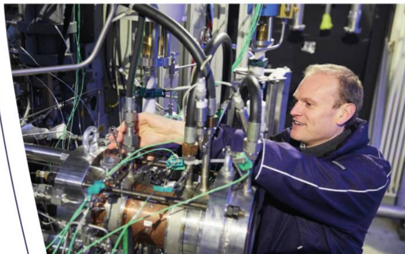
Hot run of the experimental combustion chamber model 'H' (BKH). Justin Hardi wants to contribute his knowledge of the processes in rocket combustion chambers to the development of new space propulsion technologies.
