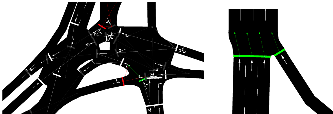
Figure 3 – Example of an intersection with network defects and thus significantly reduced traffic flows (left); Example of traffic lights at junctions of roads with different priorities. Link indices 1 to 3 with higher priority have very high potential traffic flows (right).
