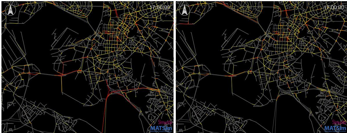
Figure 5 – Relative travel speeds at 17:00-18:00 in the base scenario (left) and in the short-term scenario with 140% capacity (right). Yellow links indicate a relative speed below 50% compared to freeflow speed; Red links indicate a relative speed below 10% compared to freeflow speed.
