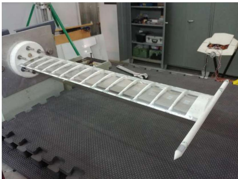
**Figure 4.** The (Pre)-Pazy wing wind tunnel model (Reproduced with permission from Drachinsky [2]; published by IACAS, 2020).
