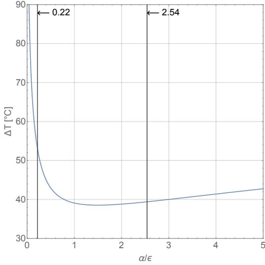
Figure 11: Difference between the hot-case sail membrane temperature as a function of  $\alpha/\varepsilon$  for LEO at the subsolar point and for deep space at 1 au solar distance.
