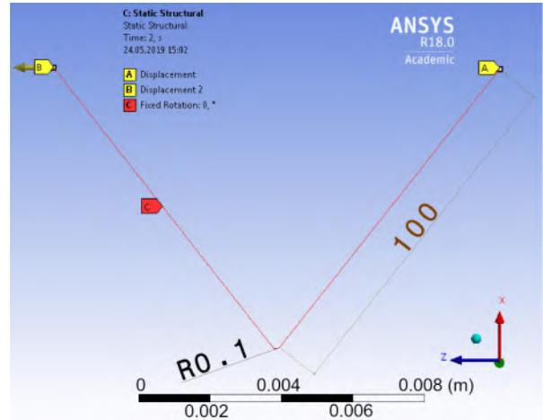
(c) Untensioned folding-line geometry and boundary conditions for FEM analysis.
