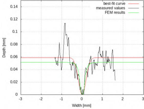
(b) Best-fit curve (red) according to Eq. (6) and FEM results (green) for the folding line (black) which was tensioned with 1.23 N ( $5.47 \times 10^6$  Pa).
