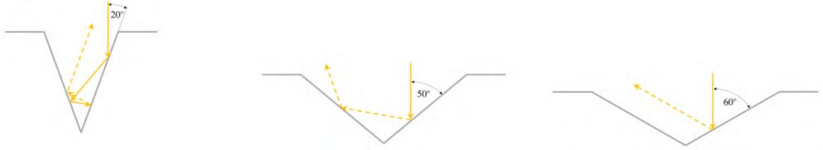
(a) Multiple reflections for small opening angles  $\psi < 90^\circ$ , here  $\psi = 40^\circ$
