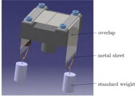
Figure 4: Sample holder for the fixation of samples with pre-tensioned folding lines.
