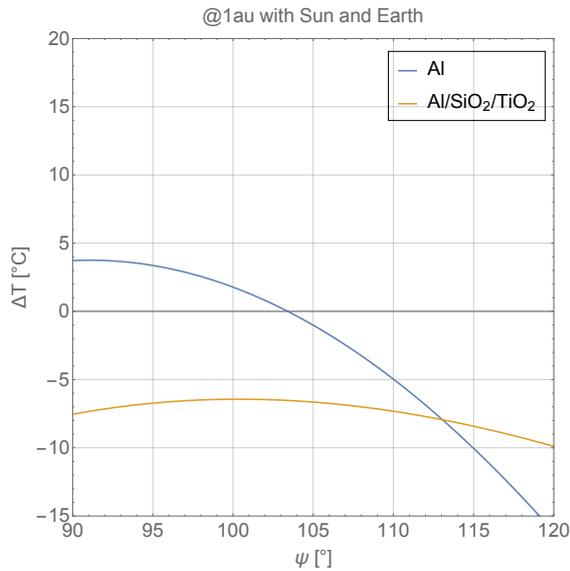
Figure 13: Temperature difference due to two reflections in the folding line for the LEO sub-solar point case. Positive values indicate a temperature increase.
