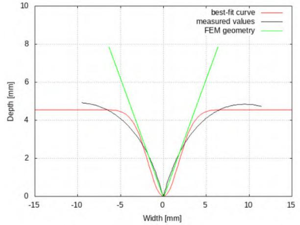
(b) Processed microscope measurements of the folding-line profile along the centerline of the sample, curve of the fit-function according to Eq. (1), and derived FEM initial geometry.
