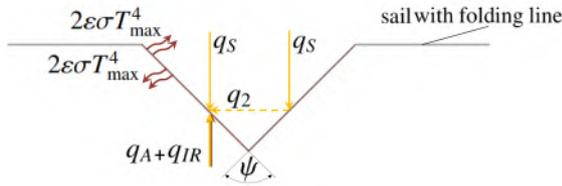
Figure 9: Heat transfer to a sail membrane with a folding line (here,  $\psi = 90^\circ$ ) facing the Sun. Transfer of heat to a point in the folding line is due to solar radiation,  $q_S$ , and reflection in the folding line,  $q_2$ . In case the sail is in an Earth orbit, additional heat transfer due to Earth albedo,  $q_A$ , and Earth infrared radiation,  $q_{IR}$ , are present.
