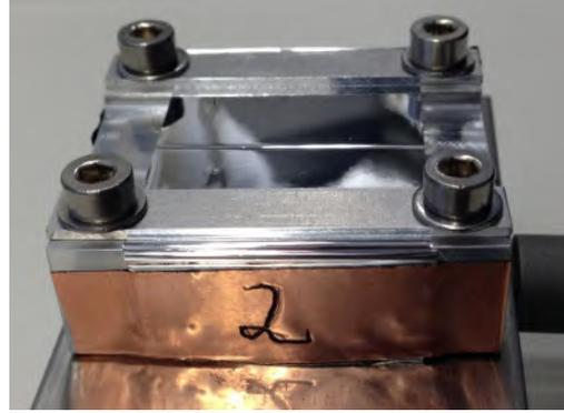
(a) Sample tensioned with a weight of 125 g fixed with the brackets on the sample holder.
