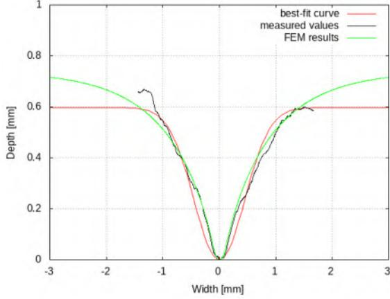
(a) Best-fit curve (red) according to Eq. (5) and FEM results (green) for the folding line (black) which was tensioned with 0.014 N ( $6.2 \times 10^4$  Pa).
