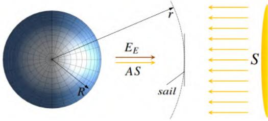
Figure 8: Illustration of the hot case for a sail in a low-Earth orbit at sub-solar point with Earth (top-of-the-atmosphere) radius  $R$ , solar sail orbit radius  $r$ , solar constant  $S$ , Earth albedo factor  $A$  and emitted Earth infrared radiation flux  $E_E$ .
