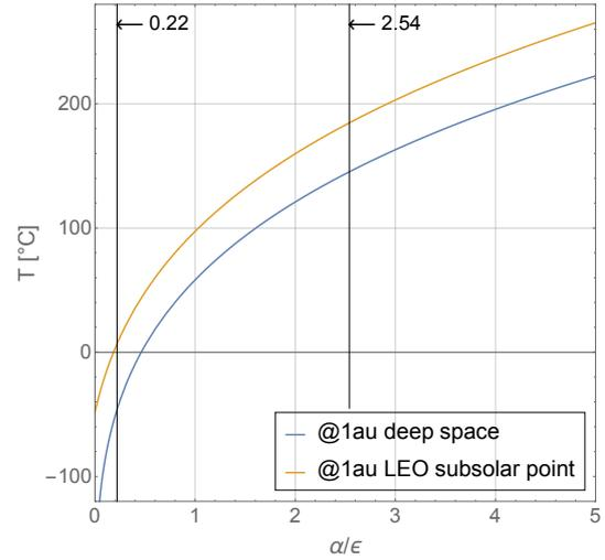
Figure 10: Hot-case sail membrane temperature as a function of  $\alpha/\varepsilon$  for deep space at 1 au solar distance and for LEO at the subsolar point.
