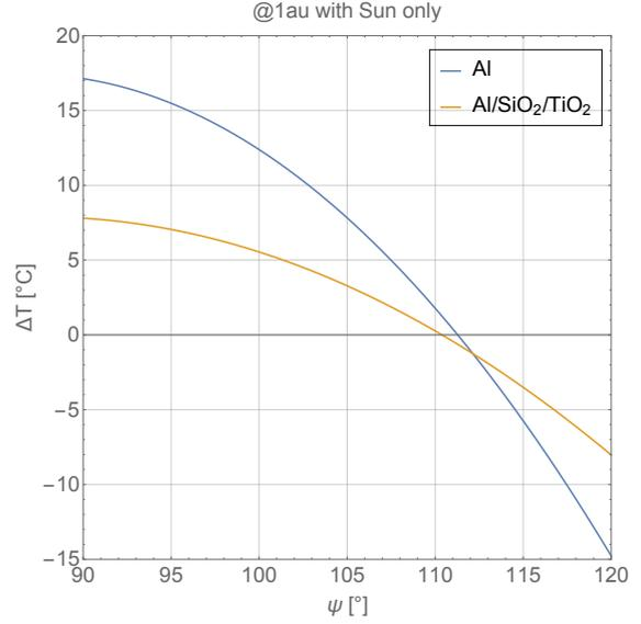
Figure 12: Temperature difference due to two reflections in the folding line for the deep space case (1 au). Positive values indicate a temperature increase.
