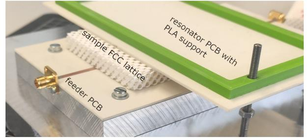
Fig. 3. System to measure dielectric permittivity consisting of an aluminium ground plate, feeder printed circuit board (PCB) with a Microstrip line, a resonator PCB with a Microstrip ring resonator and 3D printed support glued to its back and a sample of 3D printed lattice structure in FCC geometry.
