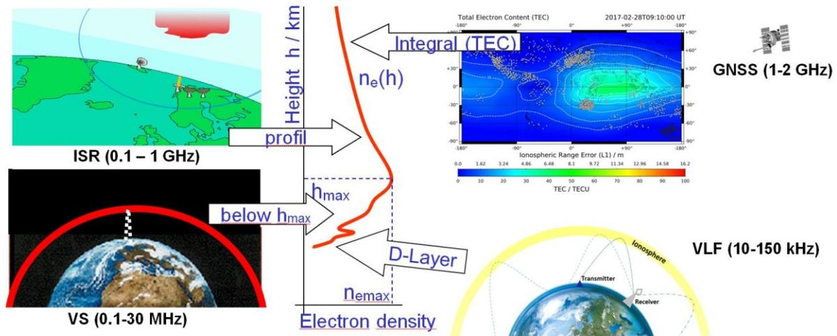
**Figure 1.** Sounding of the ionosphere with various ground based measurement infrastructures operating at different radio wave frequency bands. The combined ground based measurements supplemented by space based data can provide comprehensive information of the ionospheric profile.
