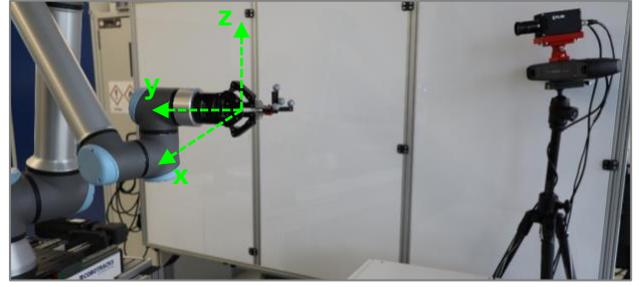
FIG 9. Test setup for validation of the tracking precision
