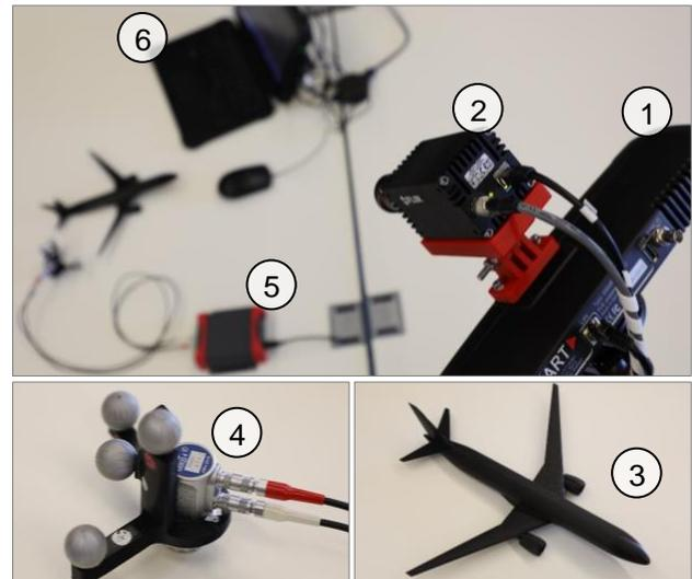
FIG 4. Setup of the hybrid tracking system
