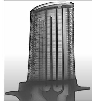
FIG 11. Turbine blade with cooling air ducts [20]
