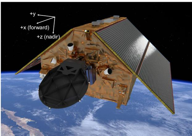
**Fig. 1** Artist's drawing of the Sentinel-6A spacecraft with the dish antenna of the advanced microwave radar and three star camera baffles on the front panel. The top panel carries three GNSS choke ring antennas for the POD and RO receivers. The three axes indicate the orientation of the spacecraft body system, with  $+x$  pointing in flight direction and  $+z$  pointing in nadir direction during nominal operations. Image credit: ESA/ATG Medialab, CC BY-SA IGO 3.0
