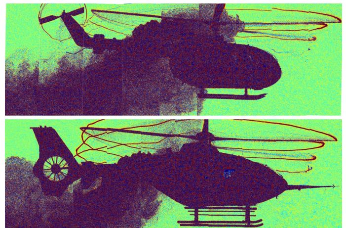
Fig. 23. Compilations of schlieren images for forward flight cases, Bo105 (top, h = 0.89 , \mu^* = 0.47 , V_x = 5.1 m s ^{-1} ) and EC135 (bottom, h = 0.87 , \mu^* = 0.76 , V_x = 9.1 m s ^{-1} ). One of the main rotor blades points forward at \Psi \approx 180^\circ .
