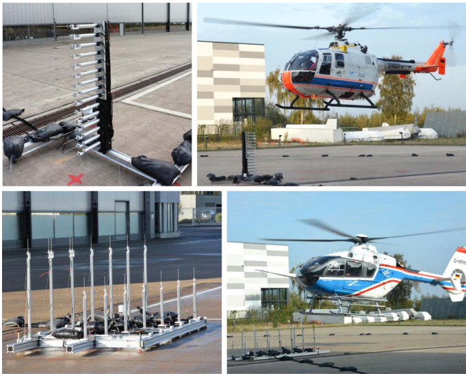
Fig. 5. Vertical array (top row) and horizontal array (bottom row) of CTA sensors.
