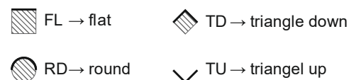
FIG. 1 BASIC OBSTRUCTIVE SURFACES FOR TRICKLING PARTICLES (BOLT) AND POSSIBLE BAR GEOMETRIES (CROSS-HATCHED).
