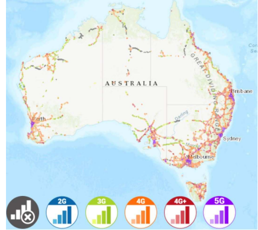
Fig. 1. The 3G/4G/5G network coverages by Telstra, which are obtained from https://www.nperf.com/en/map/AU/-/2445.Telstra/signal/ on February 21st, 2021. The network coverages by Optus and Vodafone are similar or smaller than those covered by Telstra.
