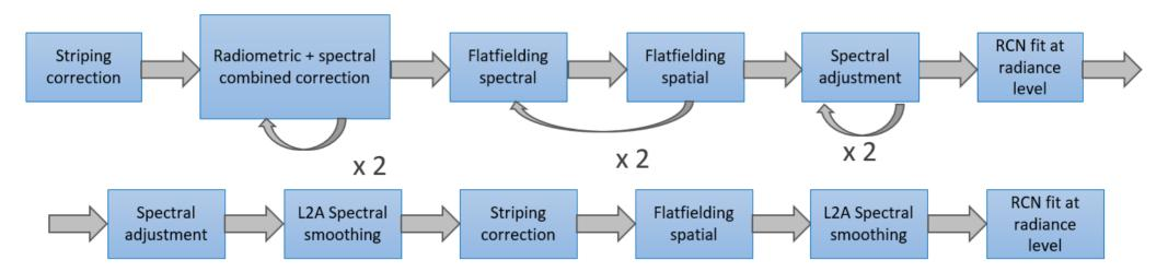
Original sequence of steps followed on first ground-to-space calibration. Newer calibration updates require simpler sequences
