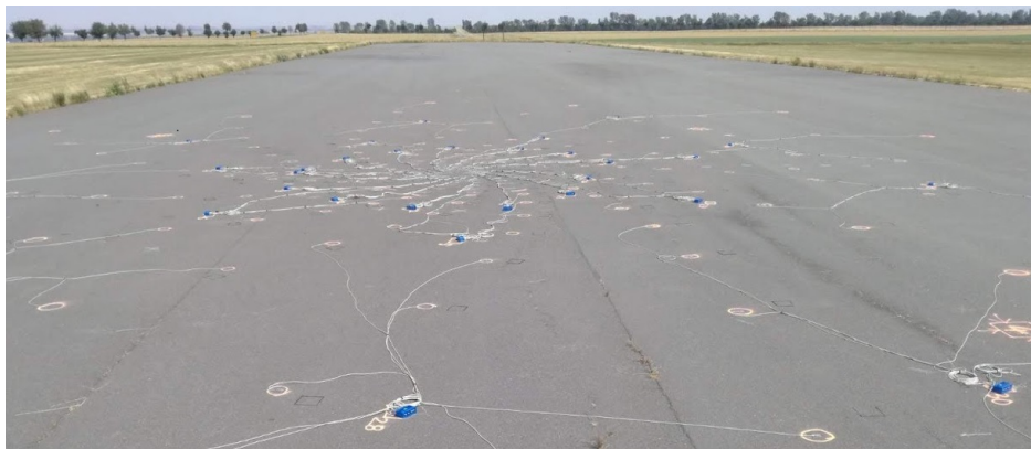
Figure 2: Set-up of the phased array on the runway for the 2019 fly-over tests.
