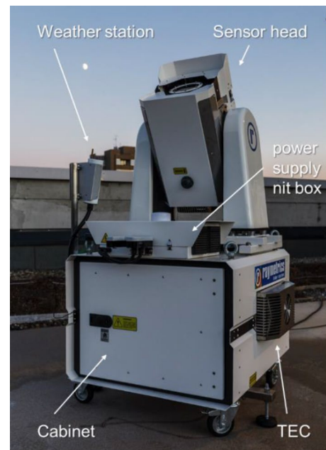
Fig. 5 Image of the Raymetrics enclosure during observation just after sunset
