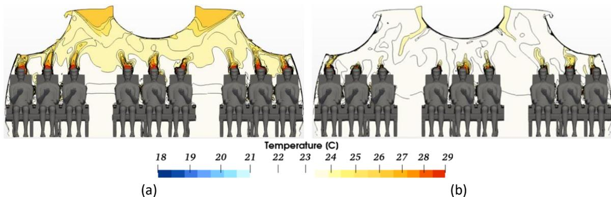
Figure 2: Comparison of temperature distribution at CDV without (a) and with (b) cooling element.
