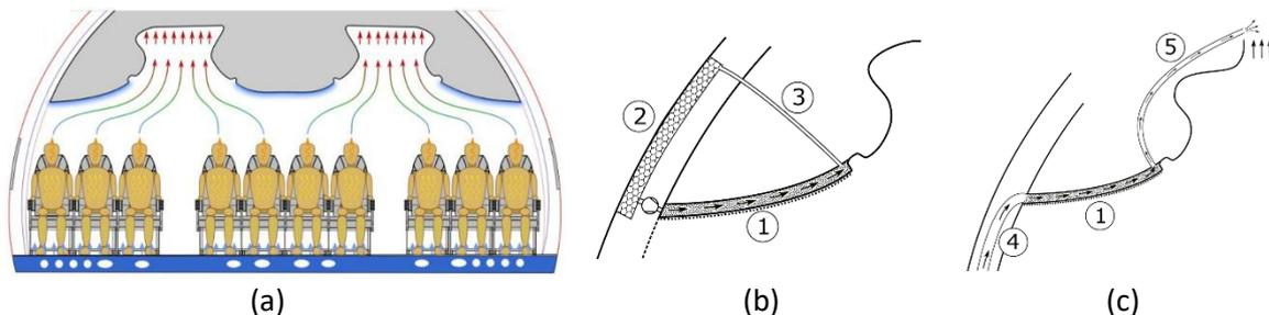
Figure 1: Integration of the cooling concept at CDV in the aircraft cabin and possible technical realisations of the element (b) as closed system and (c) as open system with the active element (1) a heat exchanger (2), the recirc pipes (3), a connection to the mixer unit (4) and an exhaust pipe (5).
