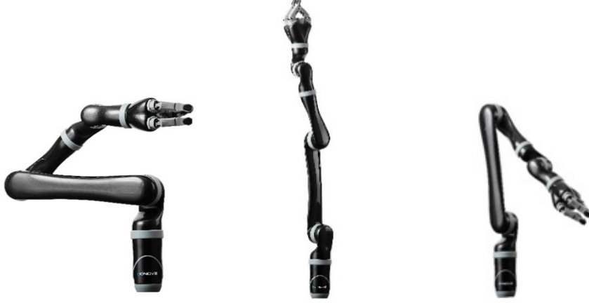
Figure 7.2.: Singular configurations of the Jaco2 arm, as given in [88]. From left to right: Wrist-over-base, boundary and wrist alignment singularity.
