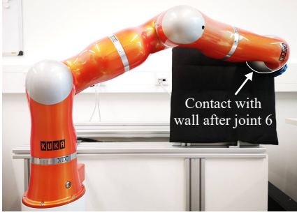
Figure 17: Setup for experiment #2b: After the sixth joint, a physical contact between the robot and its environment is enforced.
