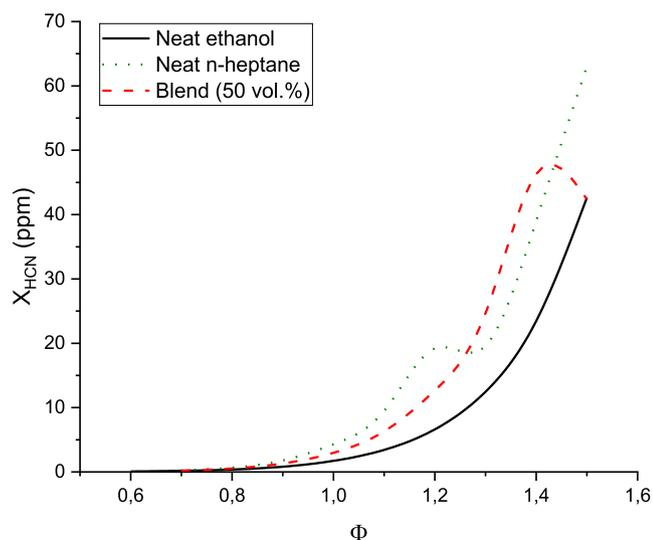
Fig. 8. Calculated peak  $X_{HCN}$  versus  $\phi$  at  $T_g = 338$  K and  $P = 1$  atm. Black solid line: Ethanol/air mixtures. Red dashed line: ethanol-n-heptane (50 vol%)/air mixtures. Green dotted line: n-heptane/air mixtures.
