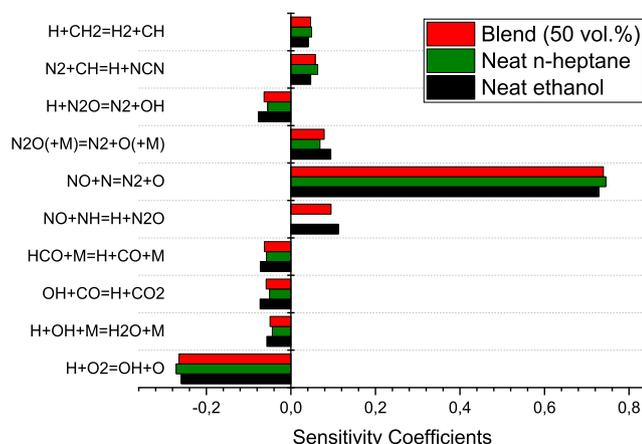
**Fig. 5.** Normalized NO sensitivity coefficients calculated at  $\phi = 1$ , HAB = 10 mm,  $T_g = 338$  K and  $P = 1$  atm for ethanol/air mixtures (black bars), ethanol-n-heptane (50 vol%)/air mixtures (red bars) and n-heptane/air mixtures (green bars). (For interpretation of the references to colour in this figure legend, the reader is referred to the web version of this article.)
