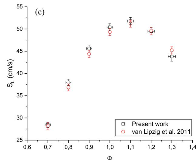
**Fig. 1.** Experimental  $S_L$  versus  $\phi$  at  $T_g = 338$  K and  $P = 1$  atm. Black squares: present work. Red circles: van Lipzig et al. [69]. Blue triangles: Sileghem et al. [86,87] (corrected according to the re-evaluation reported in [72]). (a) Ethanol/air mixtures. (b) n-heptane/air mixtures. (c) ethanol-n-heptane (50 vol %)/air mixtures. (For interpretation of the references to colour in this figure legend, the reader is referred to the web version of this article.)
