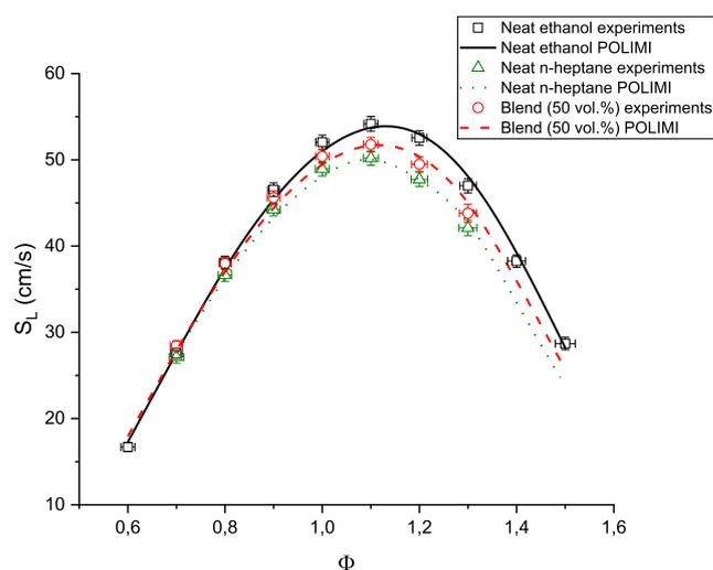
**Fig. 2.** Experimental (symbols) and simulated (lines)  $S_L$  versus  $\phi$  at  $T_g = 338$  K and  $P = 1$  atm. Black squares and solid line: Ethanol/air mixtures. Red circles and dashed line: ethanol-n-heptane (50 vol%)/air mixtures. Green triangles and dotted line: n-heptane/air mixtures. (For interpretation of the references to colour in this figure legend, the reader is referred to the web version of this article.)
