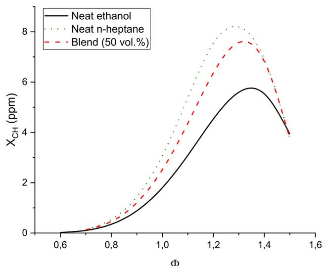
Fig. 7. Calculated peak  $X_{CH}$  versus  $\phi$  at  $T_g = 338$  K and  $P = 1$  atm. Black solid line: Ethanol/air mixtures. Red dashed line: ethanol-n-heptane (50 vol%)/air mixtures. Green dotted line: n-heptane/air mixtures.
