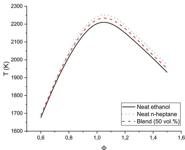
**Fig. 4.** Calculated flame temperature ( $T$ ) versus  $\phi$  at  $HAB = 10$  mm,  $T_g = 338$  K and  $P = 1$  atm. Black solid line: Ethanol/air mixtures. Red dashed line: ethanol-n-heptane (50 vol%)/air mixtures. Green dotted line: n-heptane/air mixtures. (For interpretation of the references to colour in this figure legend, the reader is referred to the web version of this article.)
