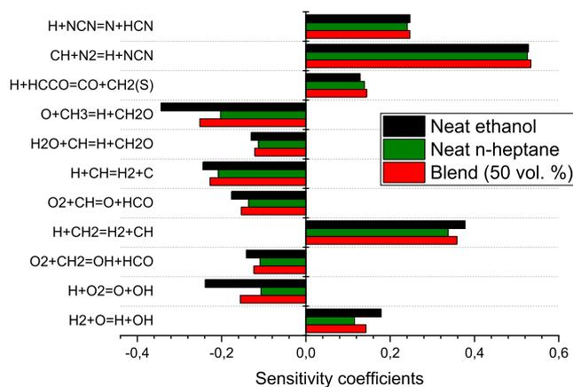
**Fig. 6.** Normalized NO sensitivity coefficients calculated at  $\phi = 1.4$ , HAB = 10 mm,  $T_g = 338$  K and  $P = 1$  atm for ethanol/air mixtures (black bars), ethanol-n-heptane (50 vol%)/air mixtures (red bars) and n-heptane/air mixtures (green bars). (For interpretation of the references to colour in this figure legend, the reader is referred to the web version of this article.)
