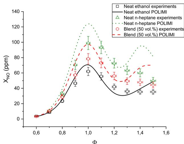
**Fig. 3.** Experimental (symbols) and simulated (lines)  $X_{NO}$  versus  $\phi$  at  $HAB = 10$  mm,  $T_g = 338$  K and  $P = 1$  atm. Black squares and solid line: Ethanol/air mixtures. Red circles and dashed line: ethanol-n-heptane (50 vol%)/air mixtures. Green triangles and dotted line: n-heptane/air mixtures. (For interpretation of the references to colour in this figure legend, the reader is referred to the web version of this article.)
