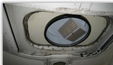
KuROS antennae on-board the SAFIRE ATR42: especially designed to validate the CFOSAT instruments
