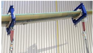
(a) Test bench.(b) Load frame.Figure 1. Experimental setup for load case Mymax by Fraunhofer IWES [8].
