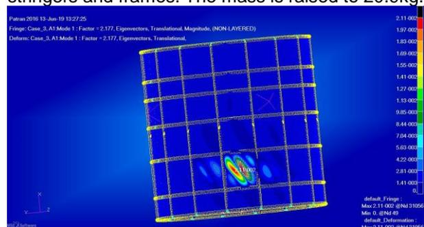
Figure 14: buckling of a cylinder with 16 stiffeners, one additional frame and a skin thickness of 1.0mm
