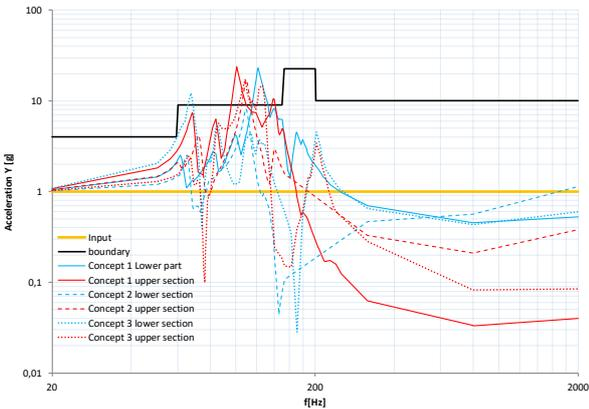
Figure 20: dynamic response in sideways direction (Y). All results are normalized to an input of 1g
