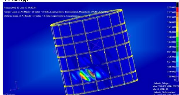
Figure 15: buckling of a cylinder with 16 stiffeners, one additional frame and a skin thickness of 1.2mm
