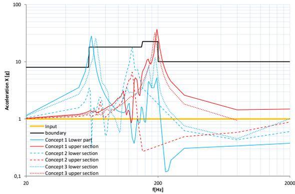
Figure 19: dynamic response in axial direction (X). All results are normalized to an input of 1g
