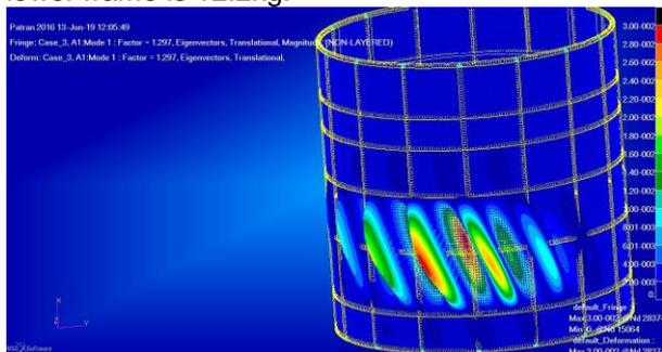
Figure 13: buckling of a cylinder without stiffener, skin thickness of 1.0mm
