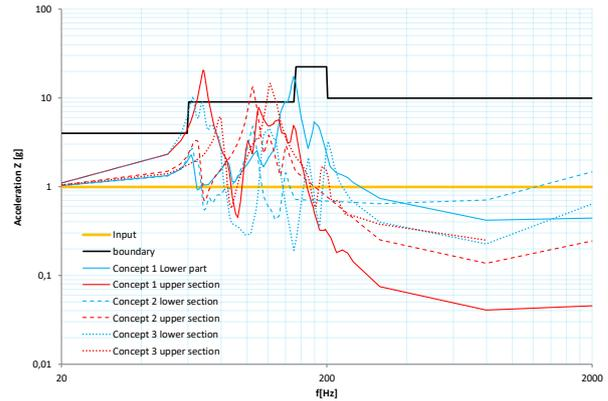
Figure 21: dynamic response in sideways direction (Z). All results are normalized to an input of 1g
