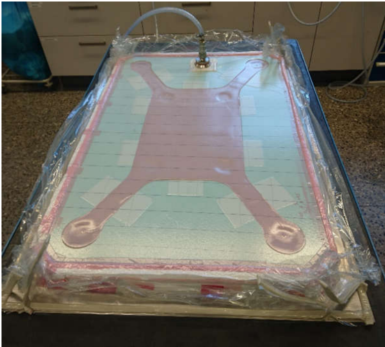
Vacuum build-up of a facesheet in the molding tool
