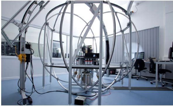
Figure 9 air bearing test stand with external Helmholtz Coil system and BIROS EM-ACS
