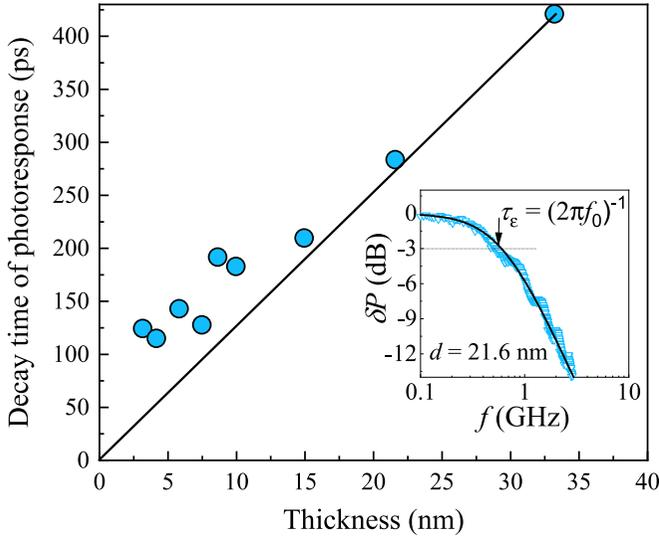
FIG. 5. Response time  $\tau_e$  vs thickness for NbN microbridges on sapphire substrates (symbols). The black line represents the linear fit  $\tau_e = 11.5d$  that corresponds to the computed phonon escape time vs film thickness. The inset shows a representative experimental  $\delta P(f)$  curve (symbols) for the sample K-8. The black curve is the fit described in the text.
