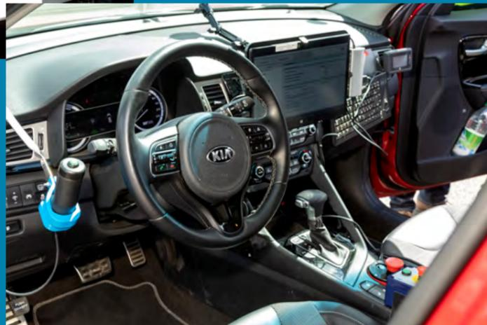
The interior of a robotic vehicle. Pre-programmed, it automatically follows a fixed route on the test site and thus simulates the surrounding traffic. Control and emergency devices enable efficient and safe testing.
