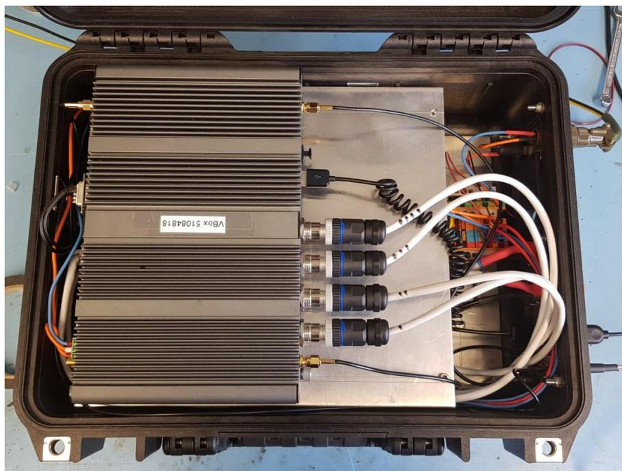
**Figure 1 - The main part of the multi-sensor unit that is installed on a shunter in the Braunschweig harbor railway. An industrial PC is visible on top, the remaining components including GNSS receiver and IMU are underneath. Not illustrated are the GNSS and communication antennas and the ABA sensors.**
