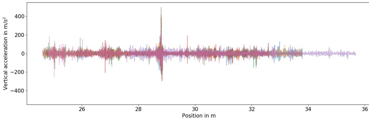
**Figure 3 - Vertical acceleration measured at multiple runs over the same track segment.**
