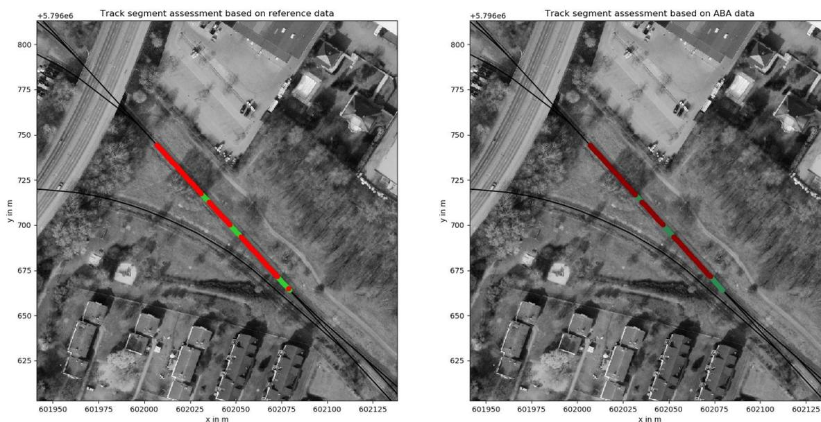
**Figure 5 - Corrugation detection based on reference and ABA data.**
