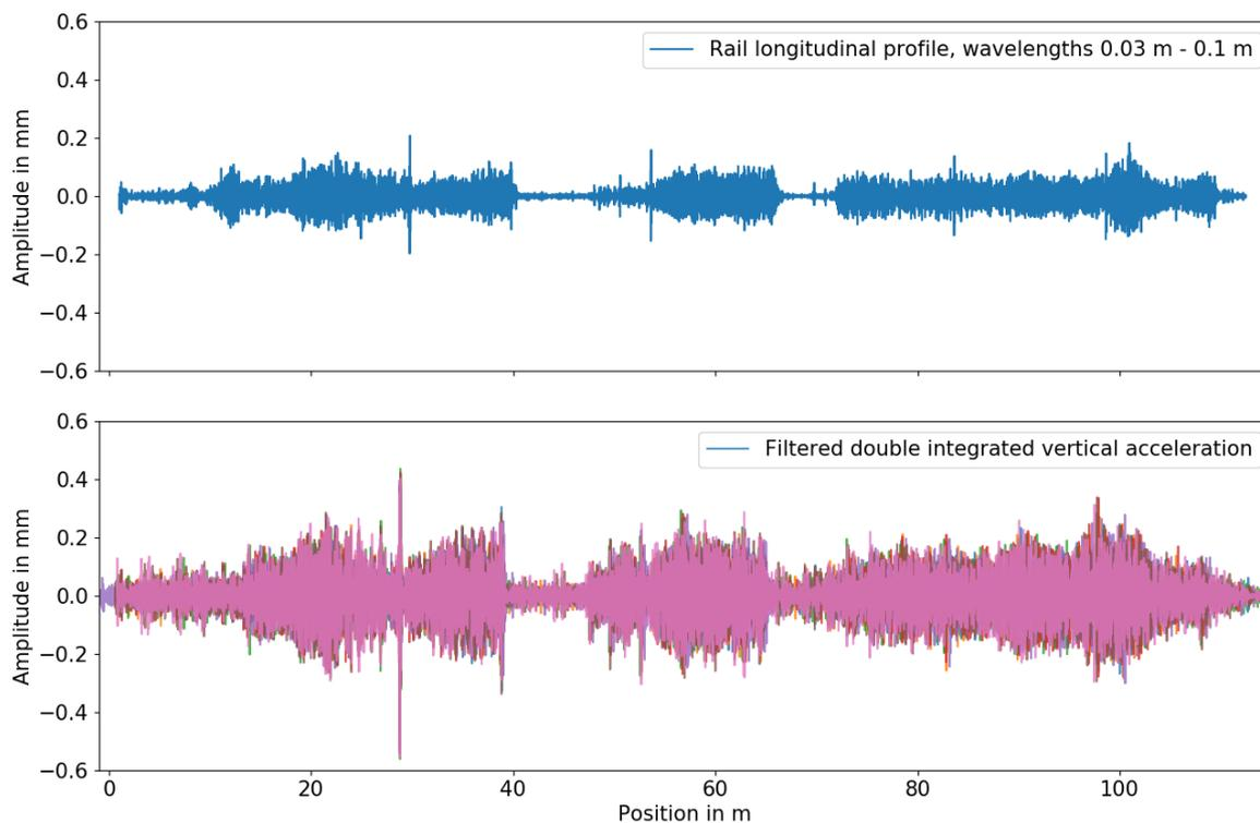
**Figure 4 - Filtered rail longitudinal profile (reference data) and filtered double integrated vertical acceleration of multiple crossings of the same track (bottom).**
