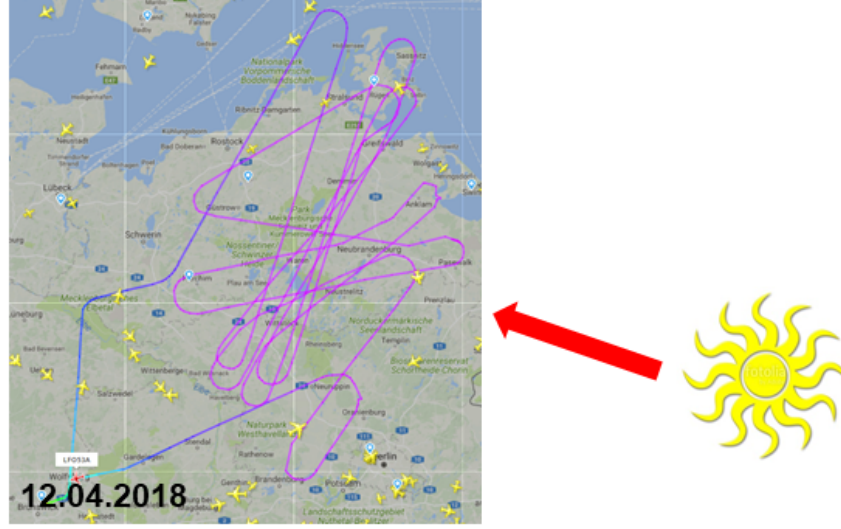
Fig. 16 Flight path with large legs perpendicular to the sun.
