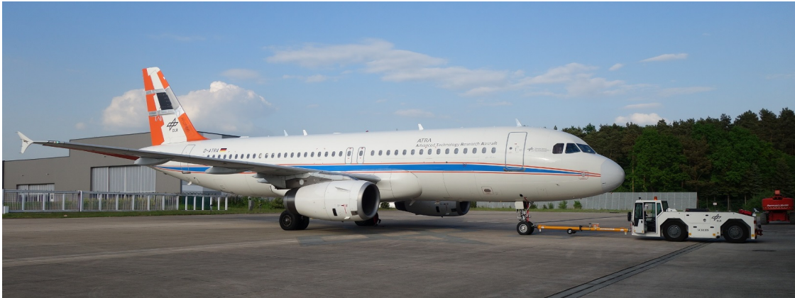
Fig. 2 DLR A320 aircraft with HLFC system installed in the VTP.
