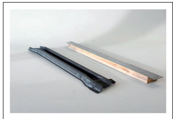
Figure 2. Reference steel component (left); generic wood–steel hybrid component (right).
