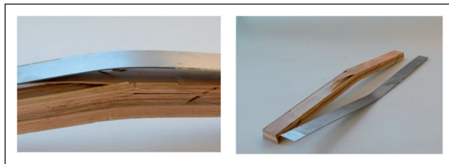
Figure 8. Three-point bending test: failed beam with steel strip (left), wooden beam and steel strip after test (right).
