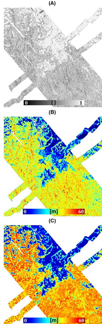
Fig. 1 – Lopé: (a) TanDEM-X volume coherence magnitude, (b) Estimated height from TDX coherence, (c) LVIS RH100 (geographic UTM coordinates).
