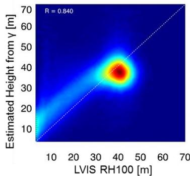
Fig. 2 – 2D histogram of the estimated TanDEM-X heights compared to the LVIS RH100.
