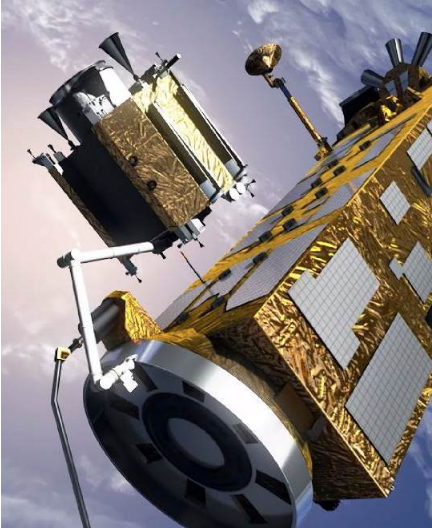
Figure 1.4.: Robotic capture scenario of the ESA e.deorbit mission: to avoid collisions with the large tumbling satellite, the orbital robot has to perform a synchronized flight during the robotic capture; the relative attitude shall be further controlled to ensure LIDAR pointing.
