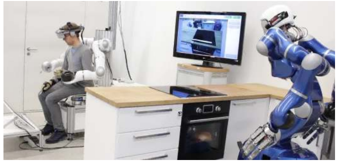
Fig. 7. Teleoperation Setup with DLR HUG (in the background) and the robotic system Justin (in the foreground)
