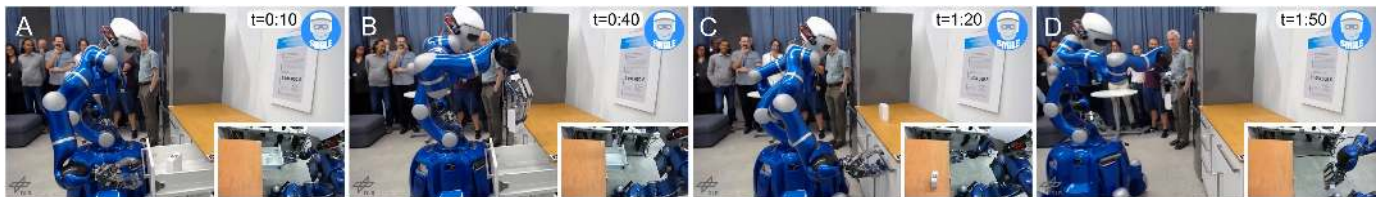
Fig. 10. Personal assistant: fetch-and-carry service of a medicine dispenser. A: opening of the drawer, B: grasping the dispenser, C: closing the drawer, D: carrying the dispenser. Execution time of this task is less than 2:00min.
