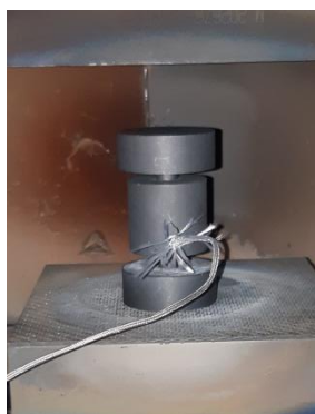
Figure 19: Die containing MgAgSb with the thermocouple controlling the temperature.
