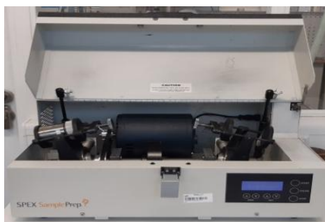
Figure 18: HEBM used during the first step of the synthesis.
