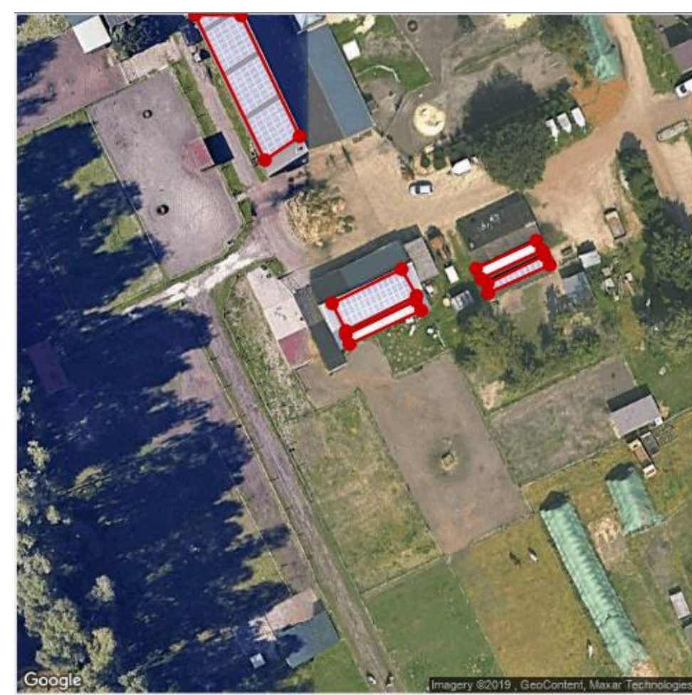
Manual identification of PV polygons in open-source tool called labelme .
