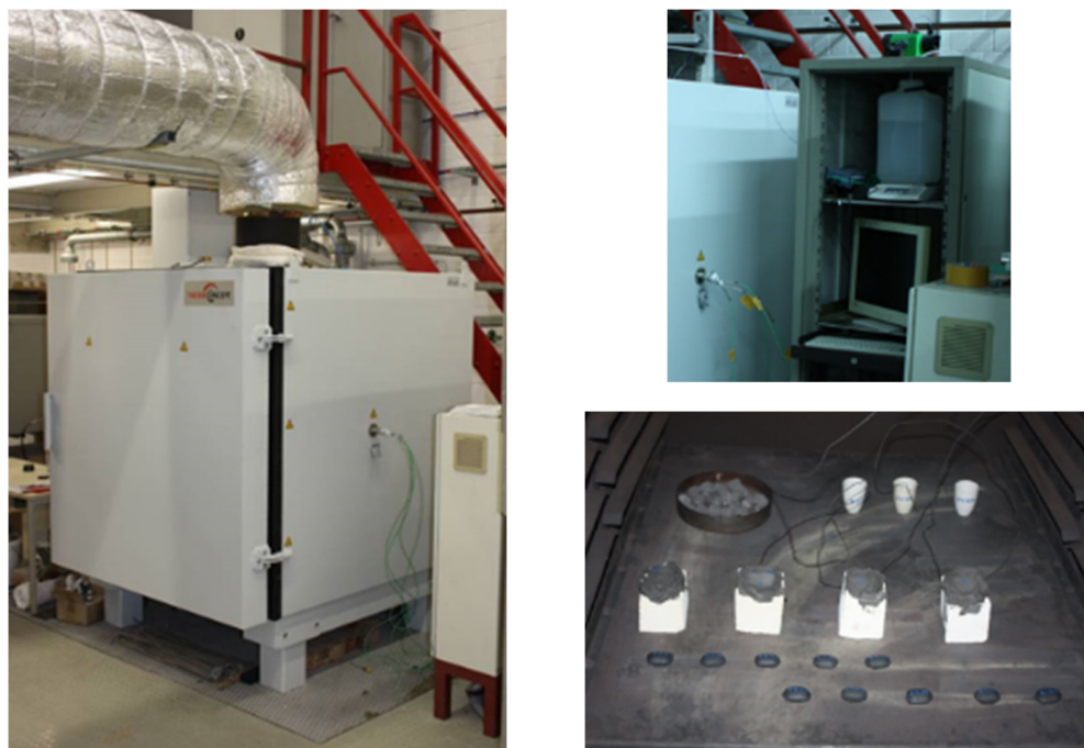
Figure S1. Air-circulation chamber furnace (left), water injection device (top right) and sample pieces and powder in the chamber with thermocouples (bottom right).
